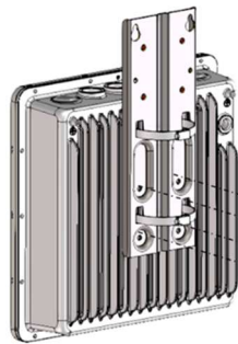
(b) Assemble the flush mount bracket with hose clamps onto the AP61
